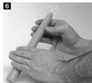
candle dipping: immerse swiftly – wait a short time (approx. 1 second) – remove swiftly – drain – cool – immerse again, and so on. If the candle has cooled down completely due to work being interrupted, the next dipping operation should last somewhat longer (about 5 seconds). Contrary to the case for beeswax candles, paraffin and paraffin/stearin candles can also be cooled in cold water (at approx. 20 °C) rather than in air. It is then important to dry the candles with a cotton cloth each time.
